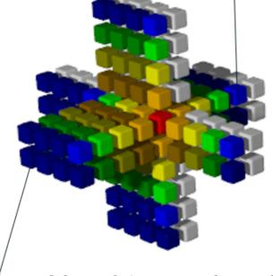
Need to read only 7 new cache lines for each iteration (vectors overlap in x-y dimensions within an iteration and in z dimension between iterations)
